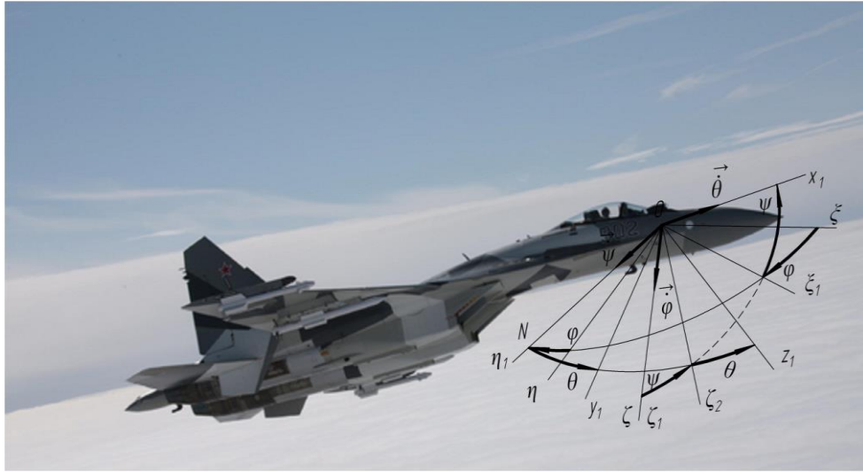
Fig. 3. Scheme angles turn of FA: \phi - angle of yaw, \psi - angle of pitch, \theta - angle of roll
